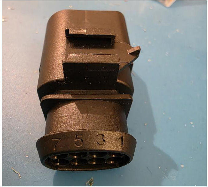
Male connector 1J0973714 with pin and rubber grommet (note that the pin number is carved on connector)
