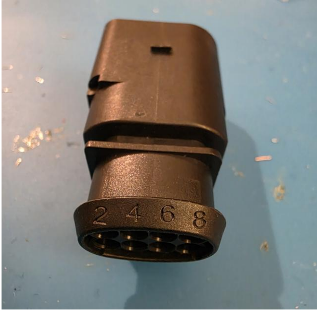
Male connector 1J0973714 with pin and rubber grommet (note that the pin number is carved on connector)
