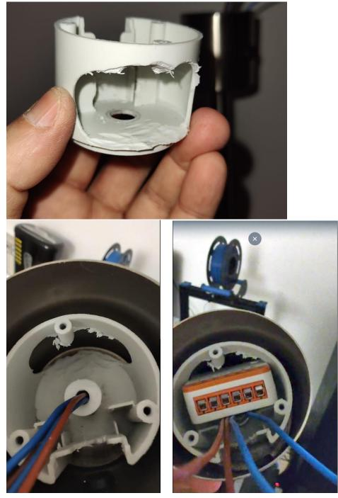
Take out the Sonoff and make the electrical connections as described in Circuit
