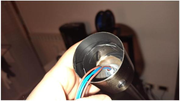
5. Carve a big hole on the plastic shell on which the bulb socket was screwed on the opposite side of the push button. How much big? Well, it has to allow the Sonoff MINI R4 to be installed diagonally, see the next picture (again the cutting like in the picture is not the best one, if you have a tool like a Dremel – I did not have one at the time I did this transformation - you can do a much better job). You have to try different times.
