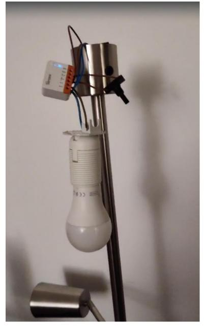
7. If everything works, **disconnect again any power source** and reassemble the Sonoff inside the plastic shell together with the black push button
